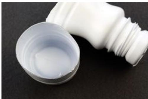
The monolayer bottles and caps are able to resist temperatures up to 95°C (© Aimplas)
